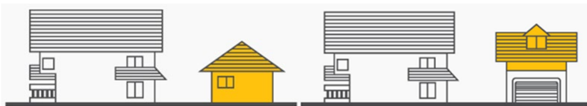
Figure 200.2: Example of a Detached ADU, include a Garden Suite (left) and a Carriage House (right).
